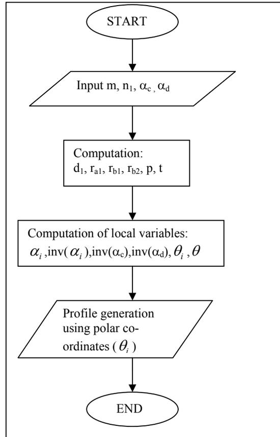
Figure 10: Flow chart to obtain asymmetric gear coordinates
