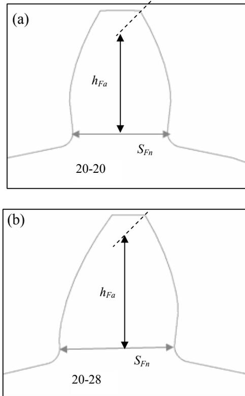
**Figure 3:** Critical sections for 20-20 and 20-28 asymmetric gear teeth
