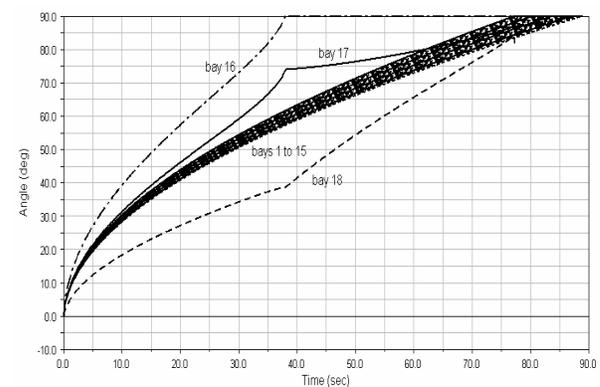
Figure 8. Angle of opening of different bays with time
