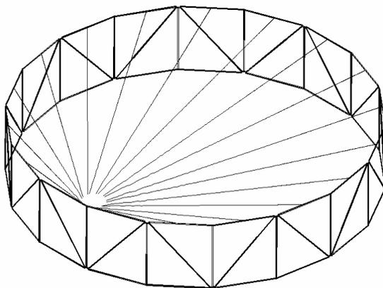
Figure 7. Path traced by the mid point of top links when they are constrained to move in a single plane
