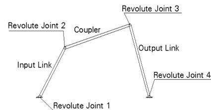
Figure 5 Four Bar Mechanism
