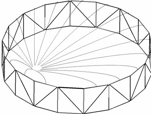
Figure 6. Path traced by mid point of the top link
