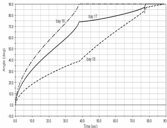
Figure 9. Angle of opening of bays 16,17 & 18 with time
