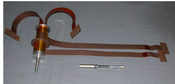
Figure 5: Flexi-print cables wound on a simulated shaft. Other end of the cable is attached to housing. Cable ends are having rigid PCB interface for connectors.
