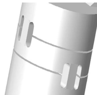
Fig 3 – Flexural hinge used in design
