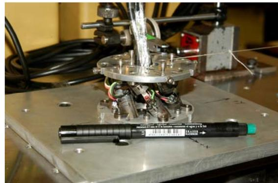
Fig 6 – Fabricated, assembled and instrumented Stewart platform sensor
