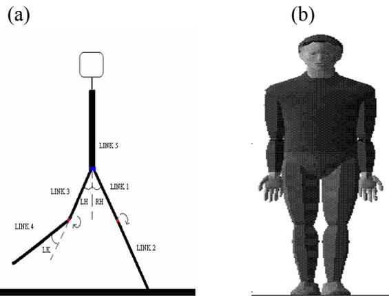
Fig. 1. Bipedal walking models (a) 5-link biped (sagittal view) (b) IGRIP humanoid (frontal view)
