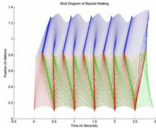
Fig. 10. Stick Diagram for Bipedal Walking (every 0.1s interval)
