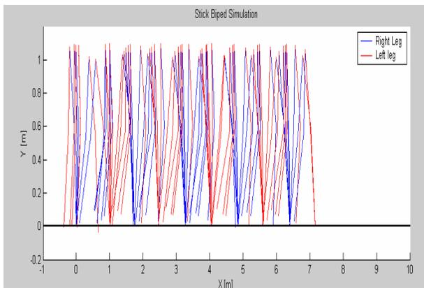
Fig. 6. Stick Picture for Bipedal walking simulations (every 0.4s interval) at  $c=4$
