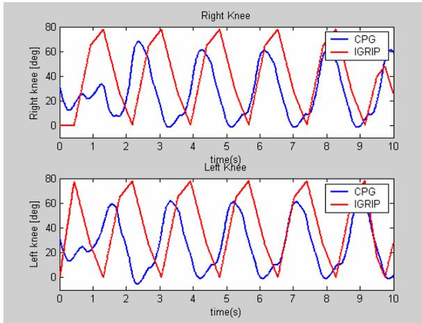
Fig. 5. Angle plot for CPG and IGRIP simulations (Right knee above and Left knee below)
