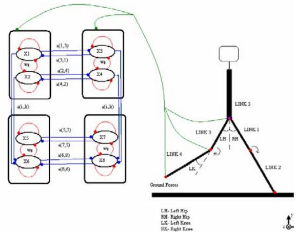
Fig. 2. Interconnections of oscillators and feedback connections.
