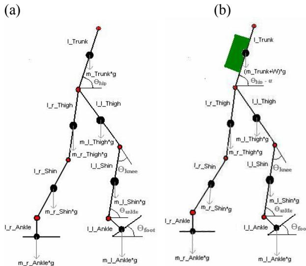
Fig. 3. Sagittal view of Bipedal Model (a) Without Load (b) With Load
