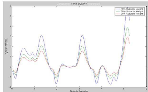
Fig. 9. ZMP Results with varying Load
