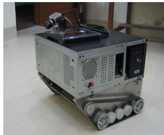
Figure 1: VITAR (VIsion based Tracked Autonomous Robot)
