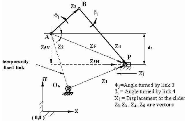
Figure 1: Off-set Five-bar slider Mechanism
