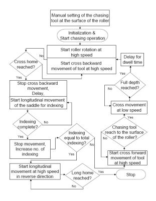
Fig.4: Flowchart of Chasing Operation
