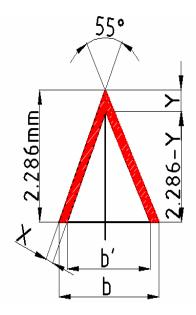
Figure 2:- chaser tool chip cross section
