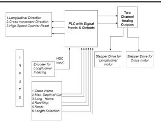
Fig. 3: Block Diagram of Electronic Controller
