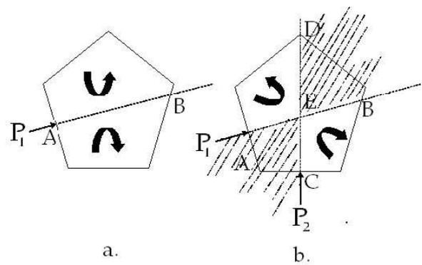
Figure 5: a. Rotational space based on a single point contact  $P_1$  at A acting at right angles to the boundary, along AB. b. Additional point contact  $P_2$  at C, along CD leading to reduction of the rotational spaces as shown. The two open shaded regions (with corners at E) i.e., AEC and BED are reduced to  $\emptyset$  spaces.
