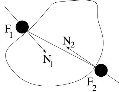
Figure 6: Geometric interpretation of the *force closure* criterion based on friction point contacts  $F_1$  and  $F_2$ .  $F_1F_2$  constitute the grasp line.  $\theta_1$  and  $\theta_2$  is below  $\theta_{min}$
