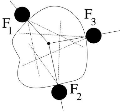
Figure 7: Geometric interpretation of the *force closure* criterion based on friction point contacts  $F_1$ ,  $F_2$  and  $F_3$ . Non-empty intersection of interior friction cones leads to force closure grasp.
