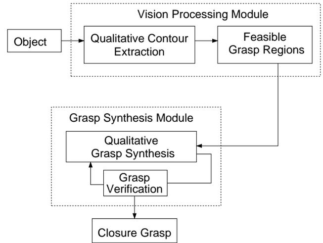
Figure 2: Framework for synthesis of vision-based closure grasps. The vision processing module exploits qualitative representation formalism for identifying the feasible grasp elements. Grasp synthesis is based on qualitative analysis and is intrinsically geometric.
