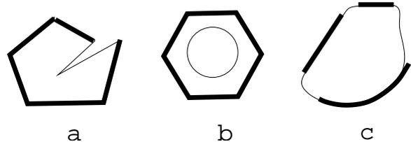
Figure 4: Feasible Grasp Regions on a. Polygon b. Hexagonal Nut and c. Circular Contour. Note that not all curve elements on the circular contour are identified as feasible, the feasible regions are based on use of minimum bounding circle defined a priori (for estimation of curvature).
