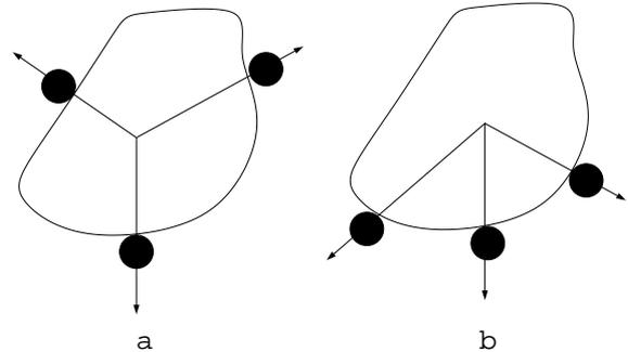
Figure 8: a. Force-closure Grasp b. Grasp that does not achieve force-closure.
