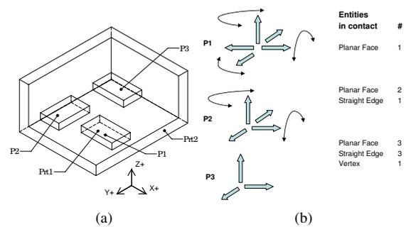
Figure 1: Relation between part positions and kinematic freedom.
