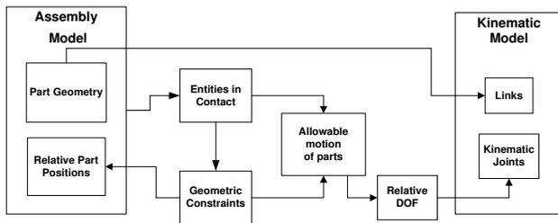
Figure 2: Relation between assembly and kinematic models.
