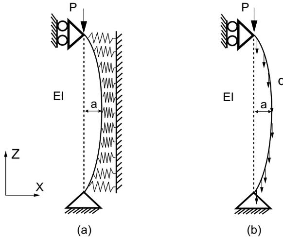
Figure 2: (a) Buckling of a pinned-pinned column on an elastic foundation. (b) Buckling of a pinned-pinned column under its own weight.
