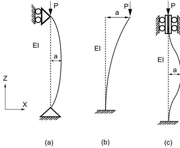
Figure 1: Buckling of columns: Case(a) Pinned-pinned (b) fixed-free (c) fixed-fixed.
