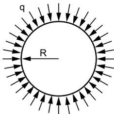
Figure 3: A uniformly loaded thin ring.
