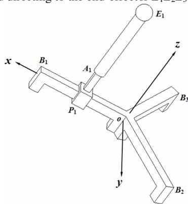
Figure 2: a Series  $PPS$  Kinematic Chain Connected with the Base
