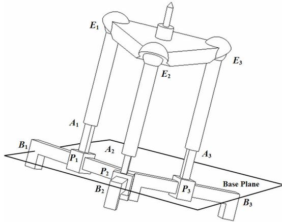
Figure 1: the Architecture of a Spatial Parallel Mechanism with 2R1T End-Effector
